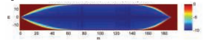
Figure 5-3 – surface elevation displacement caused by the passing vessel
