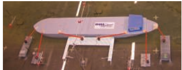
Figure 4-1 - photo of moored model vessel in the scale model.
