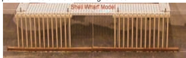
Figure 4-2 - Front of model breasting islands in the scale model.
