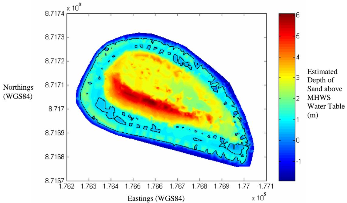
Figure 10: Estimated depth of sand available for turtle nesting above the MHWS water table elevation based on the 1994 survey data. The solid line indicates the 0.82m depth contour, which is representative of the minimum required depth for successful nesting
